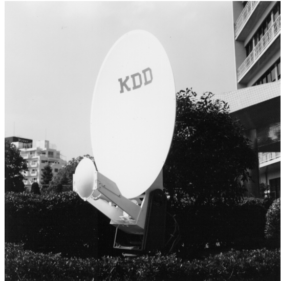
Fig. 8 1.2-m Ku-band Shaped offset Gregorian antenna for VSAT.
