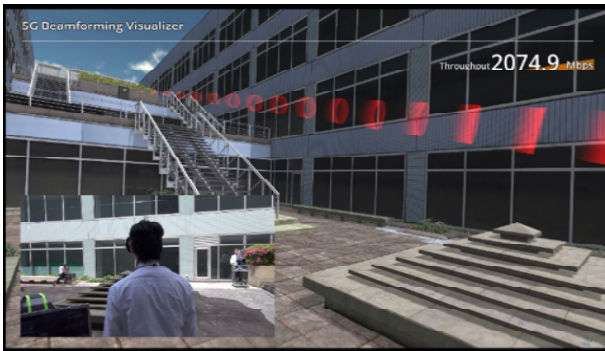
Fig. 13 Experimental trial for 3D beam tracking using the 70 GHz carrier frequency.
