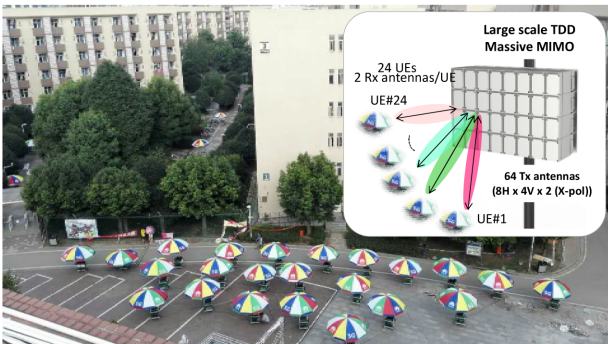
Fig. 14 Large-scale massive MIMO trial with 24 streams using below 6 GHz.
