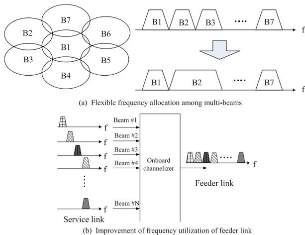
Fig. 16 Objectives of variable bandwidth channelization.
