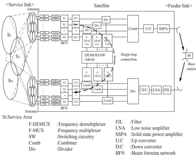
Fig. 15 Concept of single-hop connection by using OBP.
