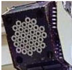
Fig. 14 ETS-VIII S-band multiple beam feeder.
