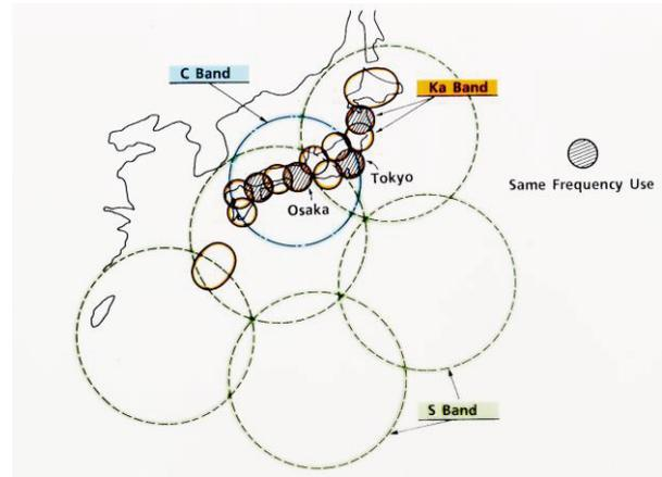
Fig. 3 Multi beam coverage of ETS-VI.
