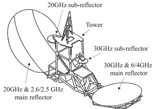
Fig. 11 Antenna system of ETS-VI.
