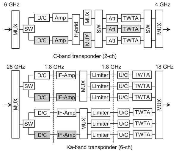
Fig. 5 Configuration of CS-2 on-board communication equipment.
