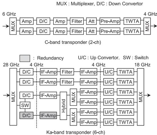
Fig. 4 Configuration of CS on-board communication equipment.
