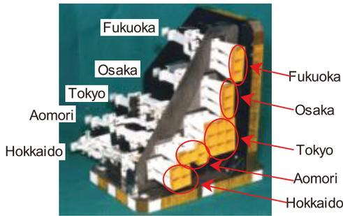
Fig. 13 ETS-VI Ka-band multiple beam feeder.
