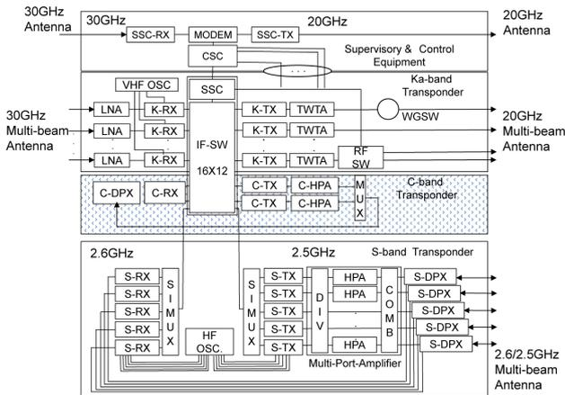
Fig. 7 Configuration of ETS-VI on-board communication equipment.
