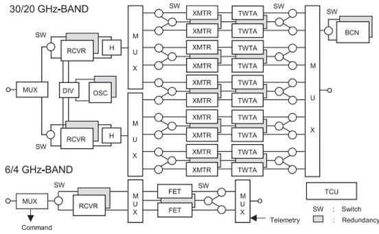
Fig. 6 Configuration of CS-3 on-board communication equipment.
