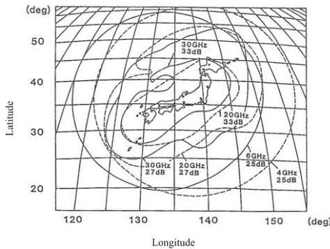
Fig. 2 Single beam coverage of CS-2.
