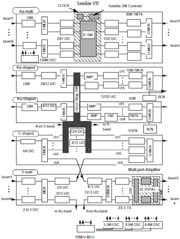
Fig. 9 Configuration of N-STAR on-board communication equipment.
