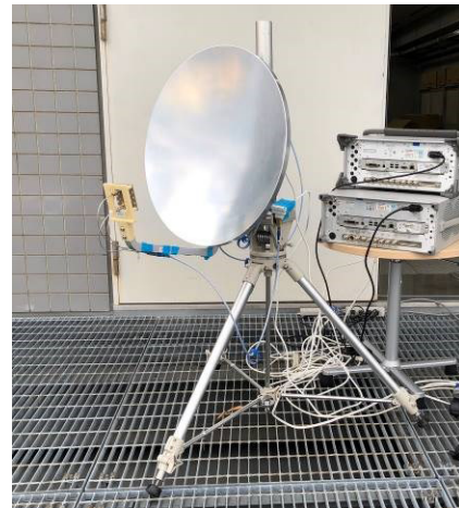
(a) Fabricated antenna receiving signals from satellites
