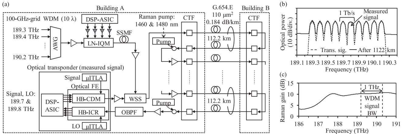
**Fig. 2** (a) Setup for field experiments over large-core low-loss G.654.E link, (b) WDM signal spectra output from WSS and after 1122-km transmission, and (c) Raman gain spectra.
