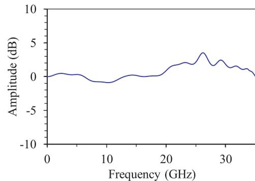
**Fig. 3** Frequency response at transmitter side of optical transponder.
