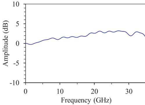
**Fig. 4** Frequency response at receiver side of optical transponder.
