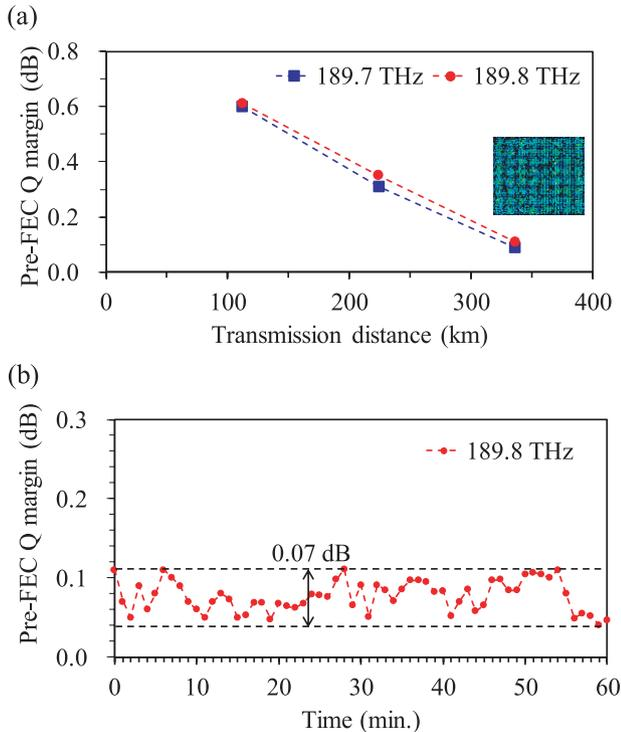
**Fig. 6** (a) Experimental result of dual-carrier 1.2-Tb/s transmission over field-deployed G.654.E fiber links and (b) stability measurements of the PDM-64QAM signal performance at 189.8 THz in WDM conditions after 336.6-km transmission.
