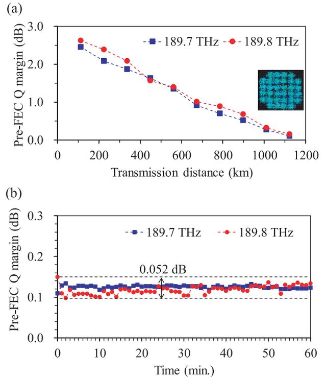
**Fig. 5** (a) Experimental result of dual-carrier 1-Tb/s transmission over field-deployed G.654.E fiber links and (b) stability measurements of dual-carrier 1-Tb/s signal performances at 189.7 and 189.8 THz in WDM conditions after 1122-km transmission.
