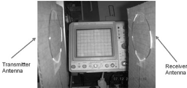
Fig. 4 Transmitter and receiver setup.
