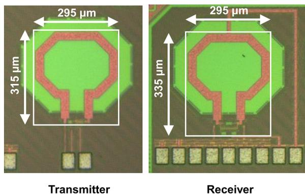
Fig. 5 Chip microphotograph for inter-chip communication.
