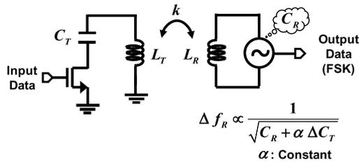
(b) Proposed FSK inductive-coupling transceiver
