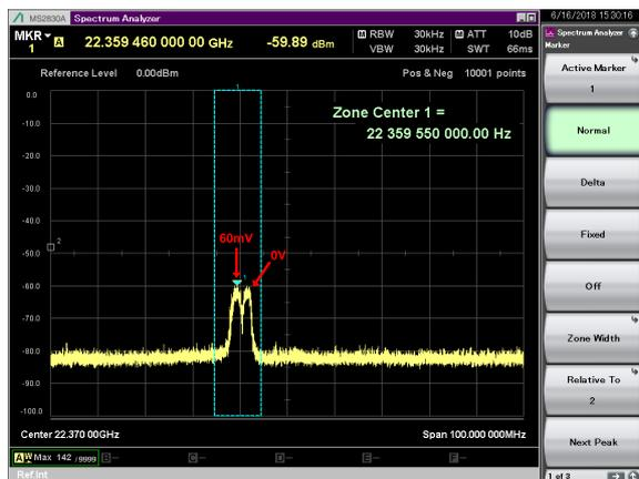
Fig. 8 Measured spectrum obtained from the chip where the transmitter input voltage is 60 mV.
