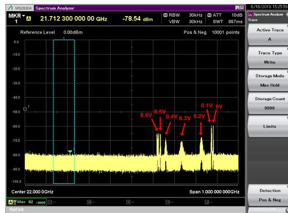
Fig. 7 Measured spectrum obtained from the chip where the transmitter input voltage changes from 0.1 V to 0.6 V.
