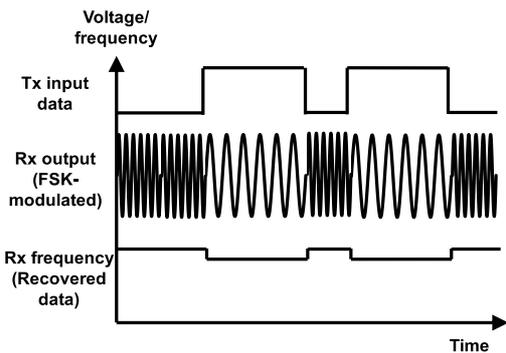
Fig. 4 Timing chart of the proposed inductive-coupling FSK communication.
