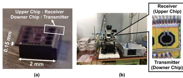
Fig. 6 Bird's eye microphotograph of the stacked chips (a) and its measurement setup (b).
