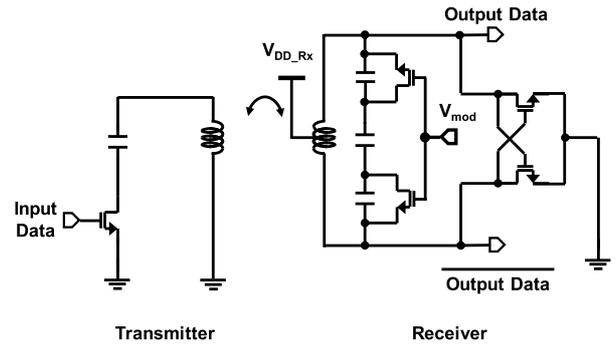
Fig. 3 Circuit diagram of the proposed inductive-coupling FSK communication.
