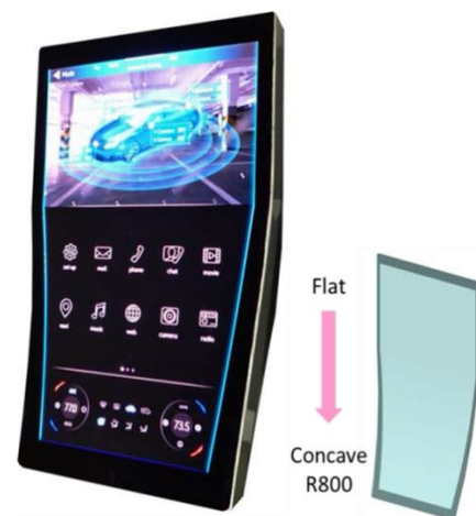
Fig. 7 A prototype of the 16.7-inch hybrid in-cell touch panel
