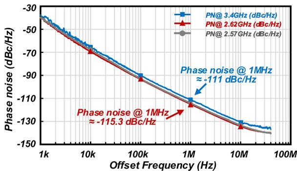
Fig. 11 Measured phase noise of the VCO at representative frequencies.
