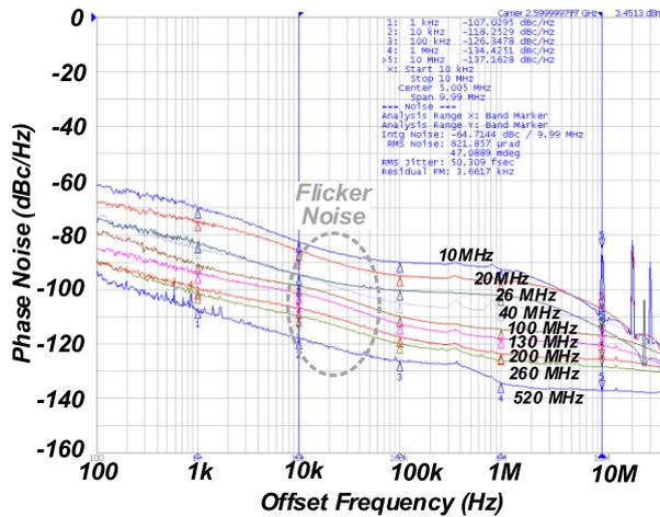
**Fig. 15** Measured injection-locked phase noise with different reference frequencies.
