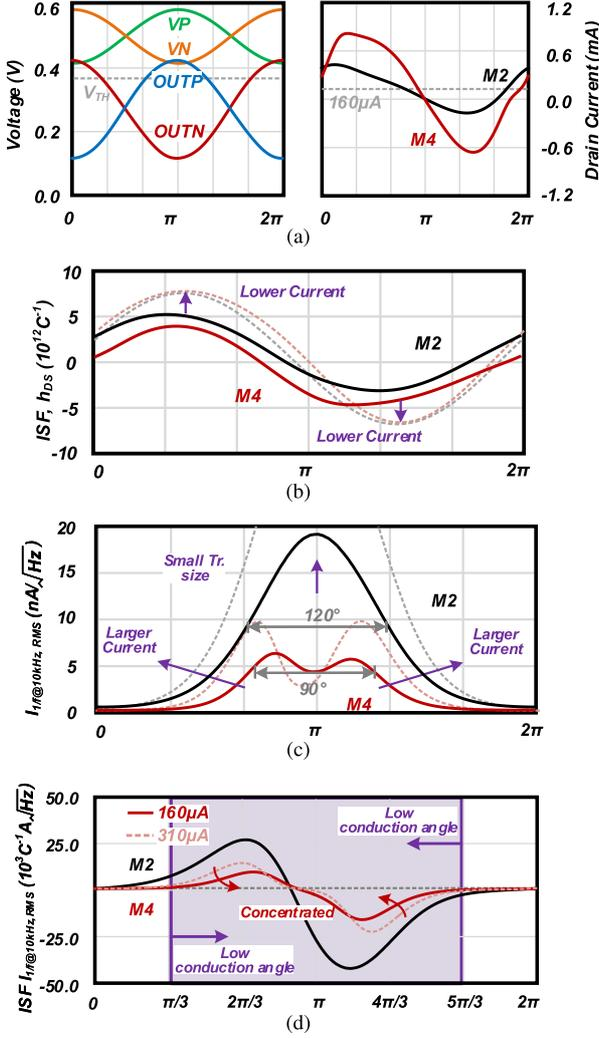
**Fig. 7** (a) Simulated waveforms of  $V_{GS}$ ,  $V_{DS}$ , and drain current  $I_D$  of transistor M2 and M4. (b) Simulated Non-normalized ISF functions of M2 and M4. (c) Modulated RMS value of flicker current noise at 10 kHz of M2 and M4. (d) Simulated effective non-normalized ISF function with different current bias (160/310  $\mu\text{A}$ ).
