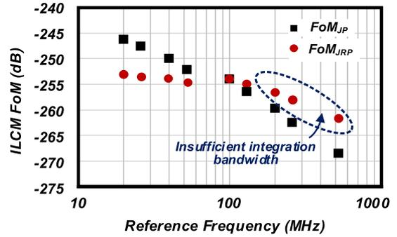
**Fig. 17** Calculated FoM with different injection reference frequencies.
