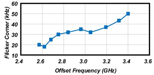
Fig. 12 Measured flicker noise corner over the frequency tuning range frequencies.
