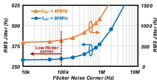
Fig. 2 Calculated jitter performance of ILCM with different VCO flicker corner.
