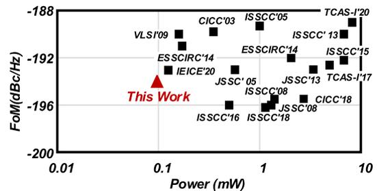
Fig. 14 The comparison of power and FoM in low-power LC-VCOs.
