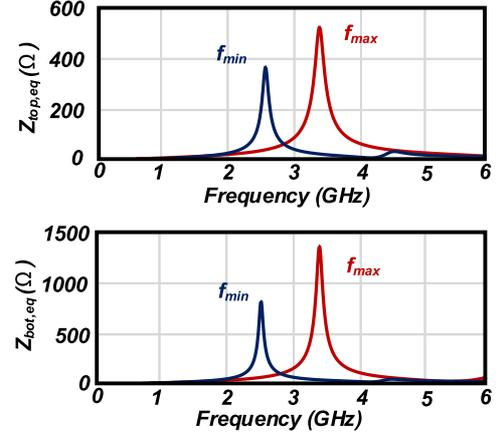
Fig. 5 Simulated tank impedance over frequency tuning range.
