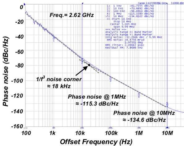
Fig. 10 Measured phase noise of the VCO at 2.62 GHz oscillation frequency.
