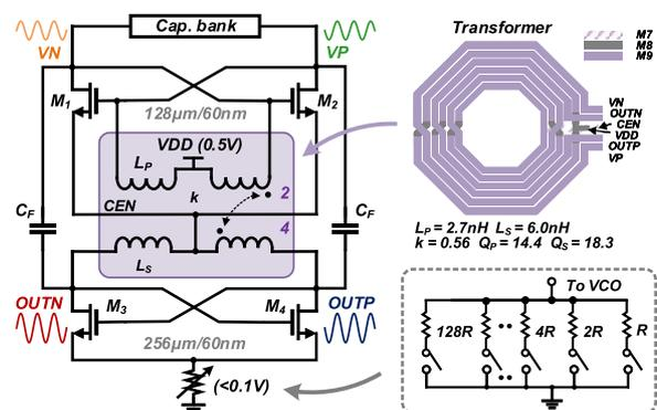
Fig. 3 Proposed ULP transformer-based VCO with flicker noise reduction.
