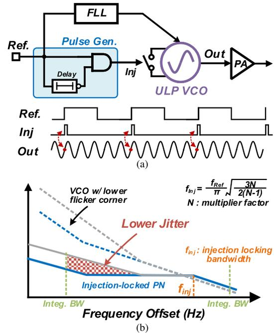
**Fig. 1** (a) Injection-locked frequency generator and its time-domain waveform during injection for frequency multiplication. (b) Lower jitter with good flicker corner.
