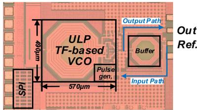
Fig. 9 Chip micrograph.
