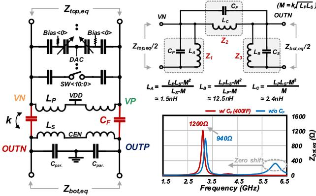
Fig. 4 Schematic of capacitor bank and equivalent model of the half transformer.
