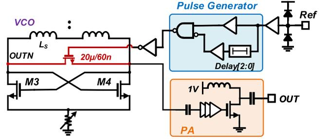
**Fig. 8** ILCM implementation with pulse generator and test buffer.
