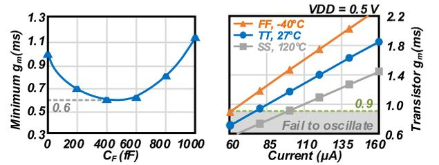
Fig. 6 Calculated minimum required  $g_{m0}$  and simulated transistor  $g_m$  versus different current bias.
