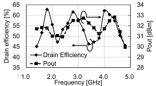
**Fig. 7** Measured frequency dependences of drain efficiency and output power at 6 dB power back-off level [17]
