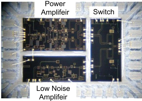
Fig. 12 Photo of fabricated GaAs RF frontend module [24]
