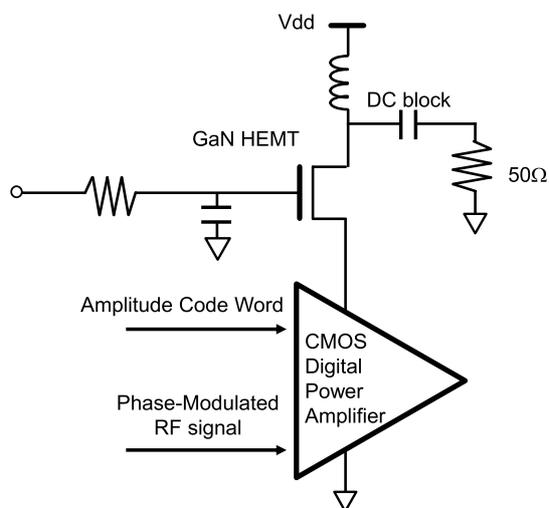
**Fig. 10** Schematic of a CMOS/GaN digital power amplifier [18]
