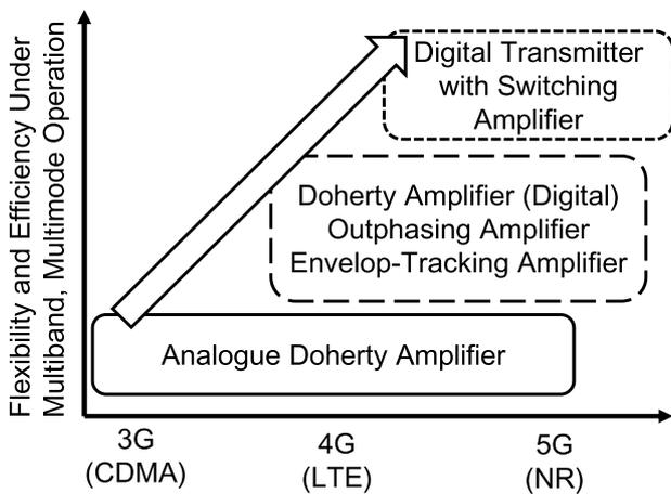
Fig. 1 BTS HPA technology trend in sub6 GHz [4]
