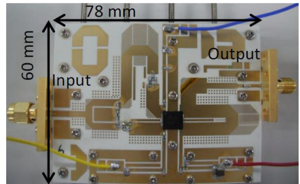
Fig. 2 Photo of wideband GaN Doherty power amplifier with frequency dependency compensating circuit (FDCC) [5]
