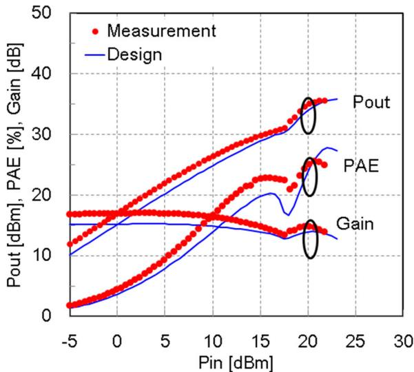
Fig. 14 Measured and simulated large-signal characteristics of the MMIC amplifier under CW operation at  $V_d = 24$  V,  $I_{dqMain} = 50$  mA/mm and  $I_{dqAux} = 0$  mA/mm. Frequency is 28.5 GHz [27]
