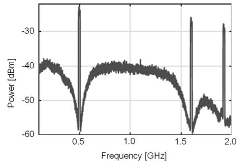
**Fig. 11** A spectrum with a full span of 2.5 GHz for the carrier frequencies of 500 MHz, 1.6016 GHz, and 1.9219 GHz with a bandwidth of 18.75 MHz [21]
