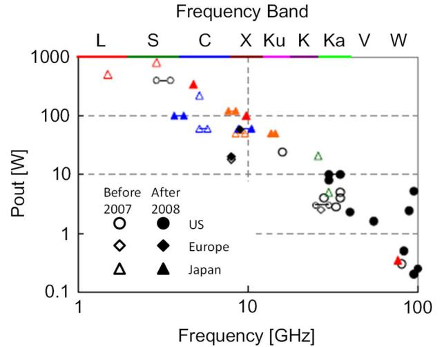
Fig. 15 State-of-the-art output power of GaN devices [31]
