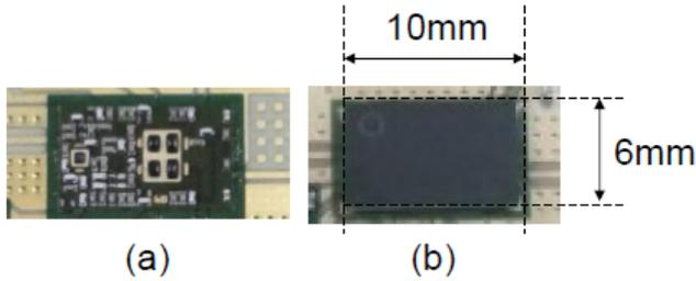
**Fig. 4** Photo of the fully-integrated 2-stage GaN Doherty power amplifier module with a compact FDCC (a) before molding and (b) after molding [16]
