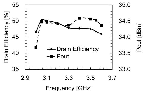
Fig. 3 Measured frequency dependences of DE and output power with ACLR of -50 dBc with DPD [5]
