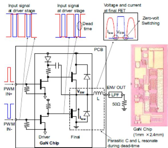
**Fig. 8** Circuit diagram of the soft-switching buck-converter and chip photo [14]
