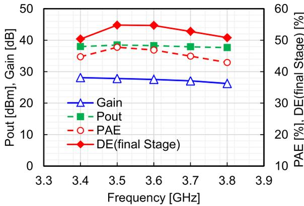
**Fig. 5** Performance of the 2-stage GaN DPA Module with a compact FDCC after molding [16]
