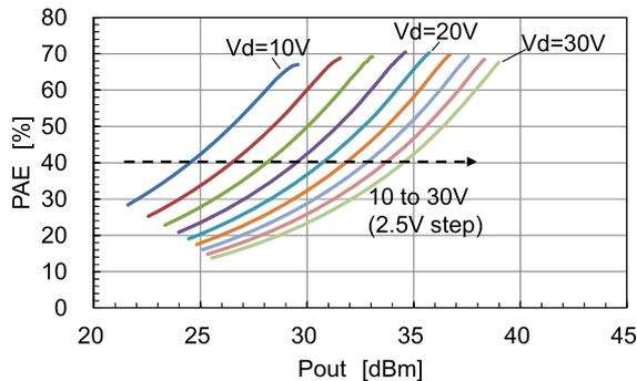
**Fig. 9** Measured PAE vs. output power of RF amplifier for ET at 3.6 GHz with various fixed power supply voltages [14]. Conversion efficiency of buck-converter is not included.
