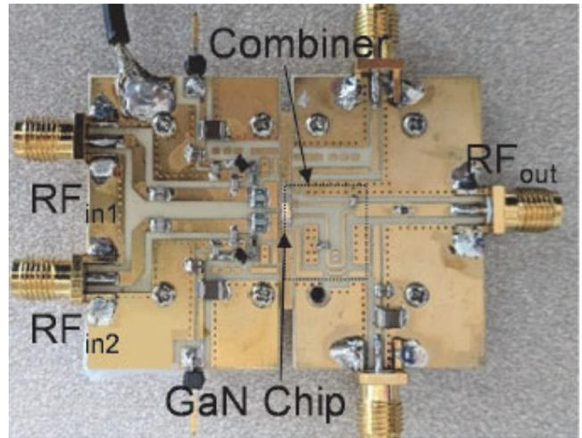
**Fig. 6** Photo of a frequency-periodic load modulated GaN power amplifier [17]
