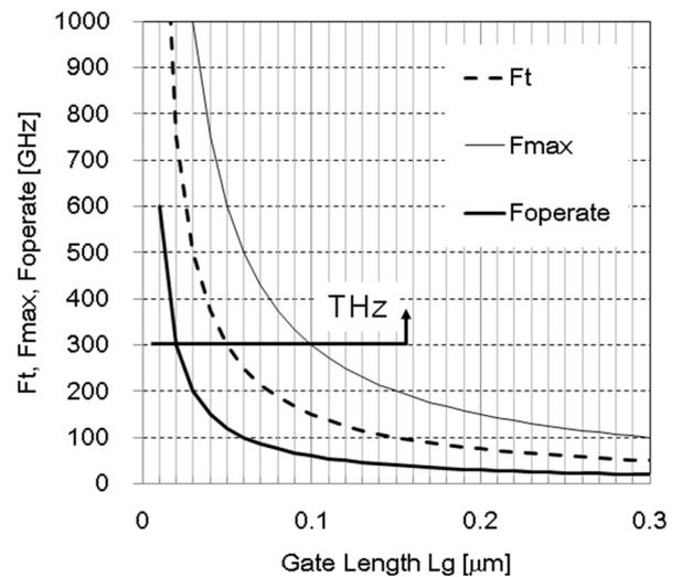
Fig. 16 Estimated  $F_t$ ,  $F_{max}$  and  $F_{operate}$  for short gate GaN FET [31]
