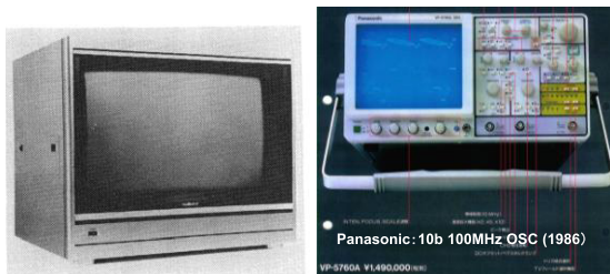
(a) MUSE HDTV receiver (b) Digital oscilloscope Fig. 4 HDTV receiver and digital oscilloscope.
