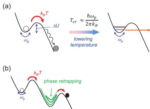
**Fig. 4** A fictitious phase particle escaping from the potential well of tilted washboard potential. (a) a crossover from the thermally activated (TA) phase escapes to the macroscopic quantum tunneling (MQT) with lowering temperatures. (b) TA escape and phase retrapping (PR) processes.
