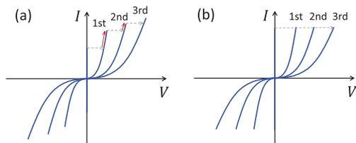
**Fig. 2**  $I$ - $V$  characteristics of IJJs, (a) a typical behavior, (b) an ideal case of IJJs where each junction has the same  $I_c$ . Red arrows in (a) represent the phase running state in the phase switched junction.
