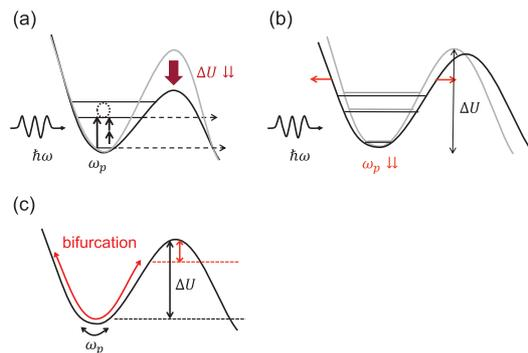
**Fig. 7** (a) Washboard potential with the reduced tunnel barrier  $\Delta U$  by irradiating microwaves. (b) Washboard potential with the expanding curvature around the bottom. (c) Bifurcation oscillation in the potential well.
