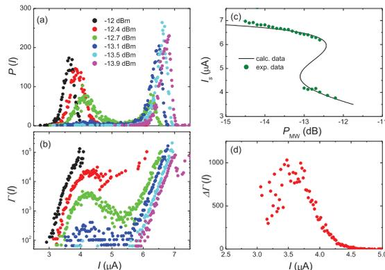
**Fig. 6** Schematic examples of (a) the microwave-resonant escapes in  $P(I)$ , (b) the corresponding switching rate  $\Gamma(I)$ , (c) the most-frequently switching current  $I_s(P_{\text{MW}})$  with a numerical calculation curve and (d) the microwave enhancement of the switching rate.
