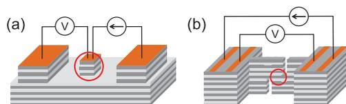
**Fig. 3** Schematics of (a) mesa-type IJJs and (b) bridge-type IJJs together with a current source and a voltmeter. Red circles represent active IJJs.
