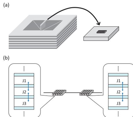
**Fig. 8** Schematics of (a) a pick-up method of a small lamella by using FIB techniques, and (b) a rough idea that two superconducting qubits with internal degree of freedom, implemented in IJJs, quantum-mechanically communicate with each other.
