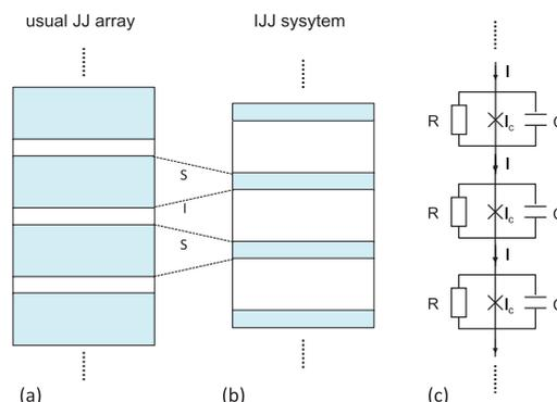
**Fig. 1** Schematics of (a) usual Josephson junction array and (b) intrinsic Josephson junction system. (c) Equivalent circuit of Josephson junction array based on the resistively and capacitively shunted junction (RCSJ) model.
