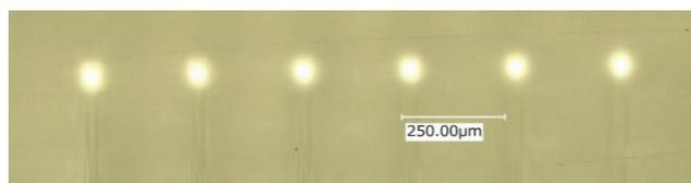
(A) Cross-section of the ending side of 3-D bent S-shaped lower 6 channels
