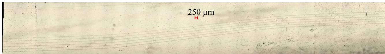
(B) Top view of the 3-D bent S-shaped upper 6-channel polymer waveguide with 250- $\mu\text{m}$  core pitch
