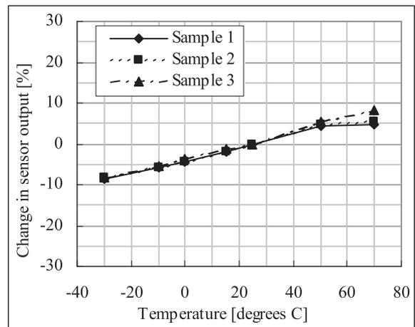
Fig. 8 Measurement result of temperature dependence of ambient light sensor output.
