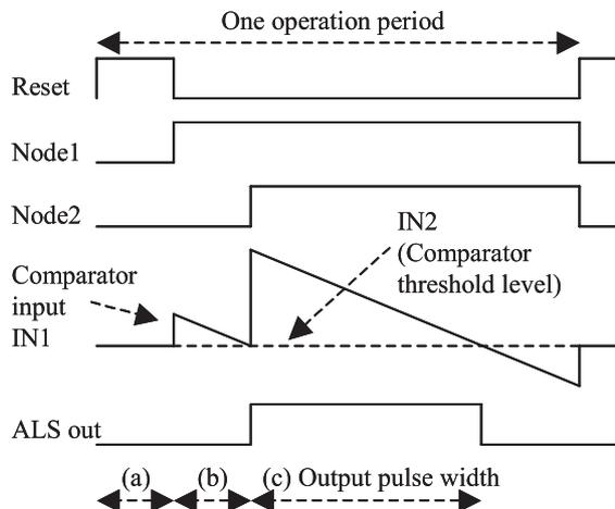
Fig. 5 Timing diagram of ambient light sensor operation.
