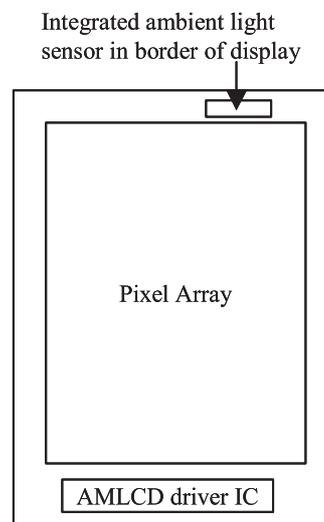
Fig. 1 Display with an integrated ambient light sensor.
