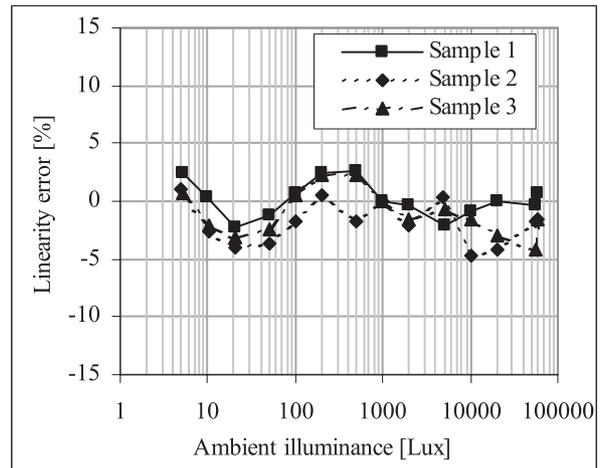
Fig. 7 Measurement result of linearity error of ambient light sensor.
