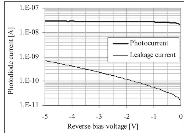
Fig. 3 Measured characteristic of a-Si Schottky photodiode.
