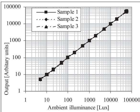
Fig. 6 Measurement result of ambient light sensor output.
