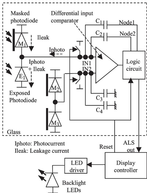
Fig. 4 Architecture of ambient light sensor and backlight control system.
