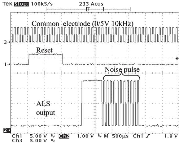
Fig. 9 Measured waveforms of an ambient light sensor of a prior technique.
