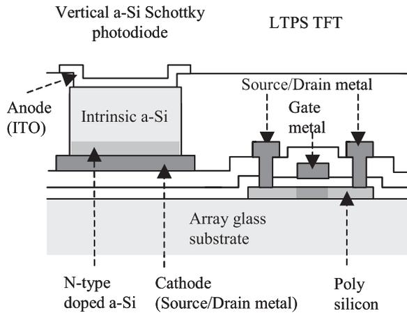
Fig. 2 Structure of vertical a-Si Schottky photodiode.
