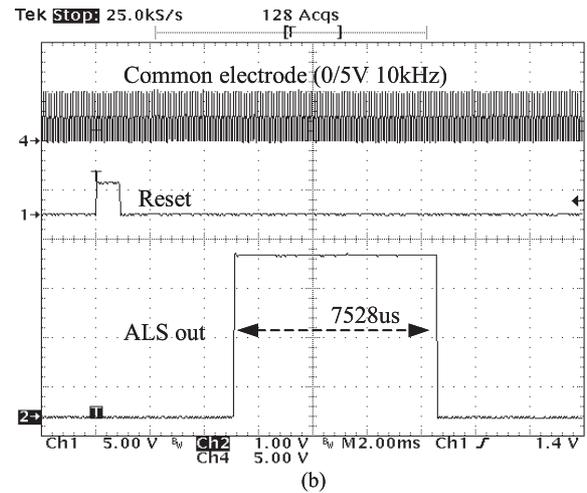
Fig. 10 Measured waveforms of the ambient light sensor introduced in this paper (a) without noise and (b) with coupling noise from common electrode.
