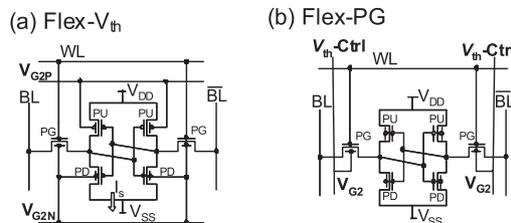
Fig. 9 Schematic illustrations of the SRAM cell.
