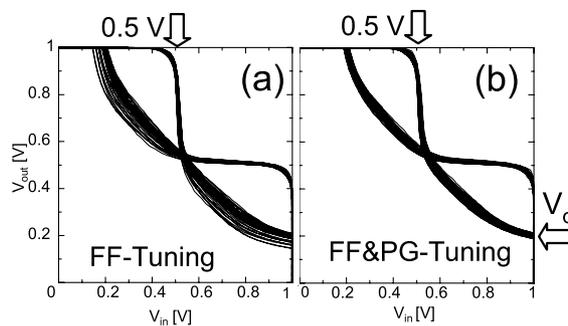
**Fig. 24** Experimental reduction of the variation by tuning (a) the bias voltage for the flip-flop, and (b) both the bias voltages for the flip-flop and the pass-gate.
