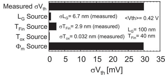
**Fig. 19**  $V_{th}$  variations due to the  $\Delta L_G$ ,  $\Delta T_{Fin}$  and  $\Delta T_{ox}$ . These values are small indicating that the dominant  $V_{th}$  variation source is the WFV.
