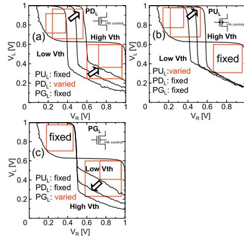
**Fig. 27** Butterfly curves of the SRAM cell with the varied  $V_{th}$  of the  $PD_L$  (a),  $PU_L$  (b), and  $PG_L$  (c) by using the IDG-FinFET.
