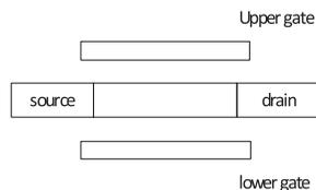
**Fig. 1** A schematic illustration of the original invention of the double-gate device.
