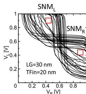
**Fig. 25** Butterfly curves for the FinFET SRAM cells. Large variation of the SNM exists.  $SNM_L$  and  $SNM_R$  are defined depending on the two different memory states. The squares in the figure show worst case  $SNM_L$  and  $SNM_R$ .
