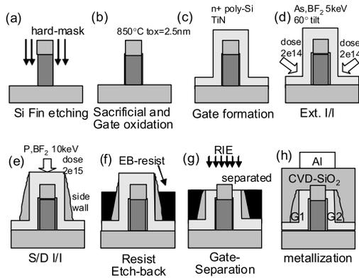
Fig. 11 Schematic device fabrication processes for the FinFET.
