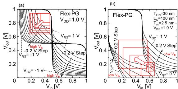
**Fig. 14** Experimental butterfly curves for the read margin (a) and write margin (b) evaluation with various  $V_{G2}$  conditions.
