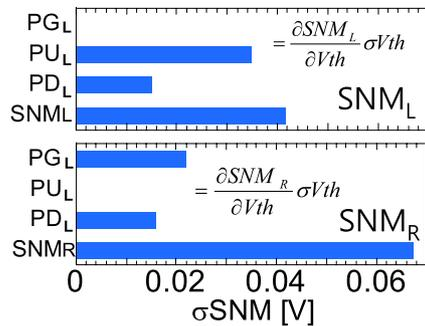
**Fig. 30** Contribution of the  $V_{th}$  variation of each transistor to the  $\sigma$ SNM.
