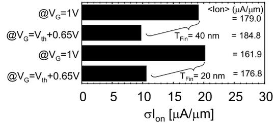
**Fig. 20** Statistical ion variation of the 100-nm-long  $L_G$  FinFETs extracted at a constant  $V_G$  ( $V_G = 1$  V) and at a constant overdrive ( $V_G = V_{th} + 0.65$  V).
