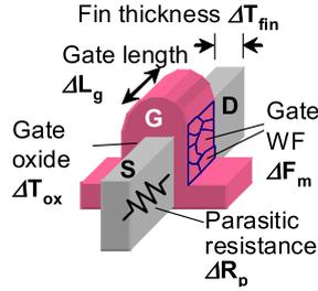
Fig. 3 A schematic illustration of the variation sources in the FinFET.
