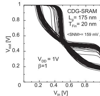
**Fig. 21** Experimental butterfly curves of the common-DG FinFET SRAM cell.
