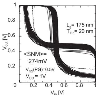
**Fig. 22** Experimental butterfly curves of the Flex-PG FinFET SRAM cell.
