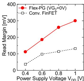
**Fig. 16** Comparison of the read margin as a function of the supply voltage.
