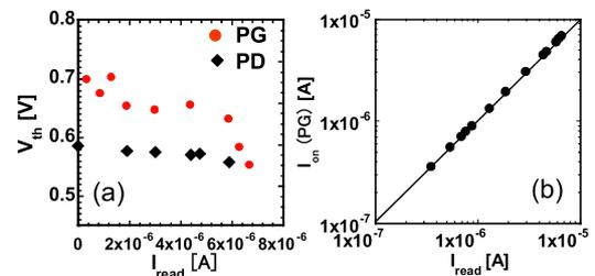
**Fig. 28** (a) Relationships between the  $I_{read}$  and the  $V_{th}$  of the PG and PD. (b) Relationship between the  $I_{read}$  and the  $I_{on}$  of the PG. The read current is correlated with the  $V_{th}$  of the  $PG_L$ . A one to one relationship was revealed between the  $I_{on}$  of the PG and the  $I_{read}$ .
