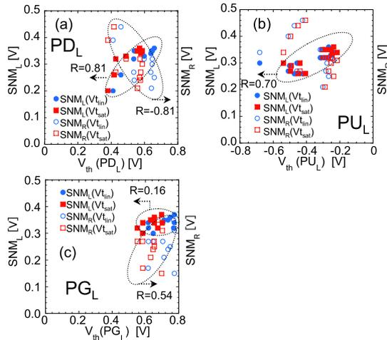
**Fig. 26** Relationship between the SNMs and the  $V_{th}$  of the  $PD_L$  (a),  $PU_L$  (b), and  $PG_L$  (c).
