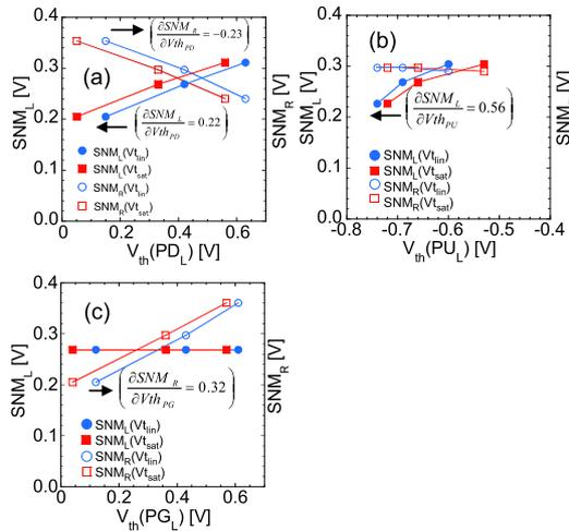
**Fig. 29** The measured SNM as a function of the  $V_{th}$  of the  $PD_L$  (a),  $PU_L$  (b), and  $PG_L$  (c) taken by controlling the second gate of the IDG-FinFET. The slope represents sensitivity.
