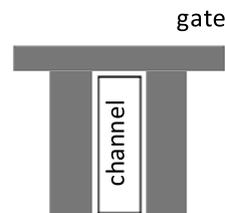
**Fig. 2** A schematic illustration of the vertical channel double gate device.
