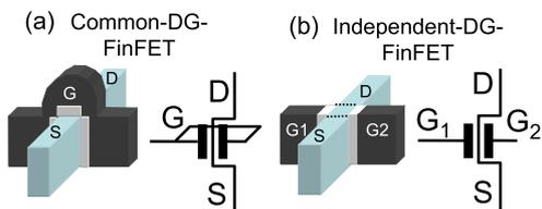
Fig. 7 Schematic illustrations of the FinFET; (a) common DG FinFET, (b) independent DG FinFET.
