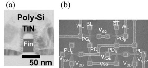
Fig. 12 A cross sectional TEM image of the FinFET (a) and a plane SEM image (b) of the SRAM cell.
