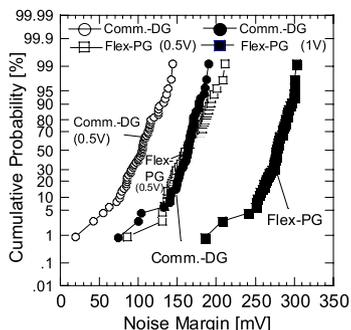
**Fig. 23** Noise margin distributions of the CDG and Flex-PG cell during 1 V and 0.5 V operation.
