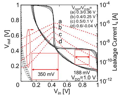
Fig. 13 Experimental butterfly curves and short circuit currents of the Flex- $V_{th}$  cell as a function of various biasing conditions.
