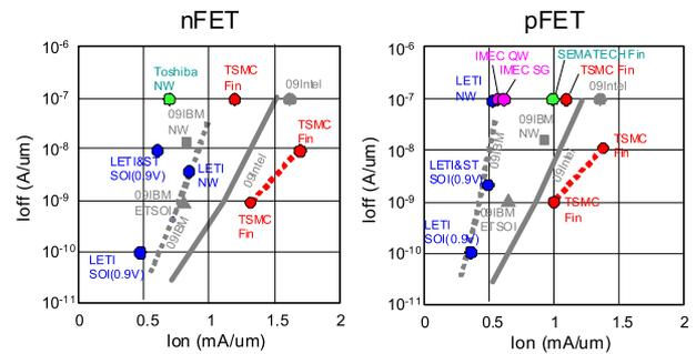
Fig. 5 Ion-Ioff plot of the scaled transistors; (a) nFET, (b) pFET.
