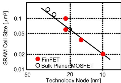
Fig. 6 The reported SRAM cell size as a function of the technology node.
