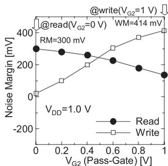
**Fig. 15** Experimental noise margins as a function of the  $V_{G2}$  for the pass gate.
