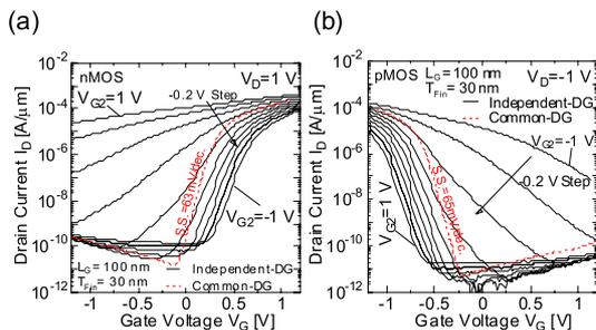
Fig. 8  $I_D$ - $V_G$  characteristics of the FinFETs; (a) nMOS, (b) pMOS.
