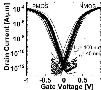
**Fig. 17**  $I_D$ - $V_G$  characteristics of the TiN Metal-Gate FinFET.
