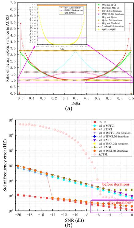
**Fig. 2** (a) Ratio of asymptotic variances of different algorithms to ACRB before and after iteration ( $SNR = 0, N = 1024$ ); (b) comparison of frequency estimation errors of different algorithms under different SNRs before and after iteration ( $N = 1024$ ).
