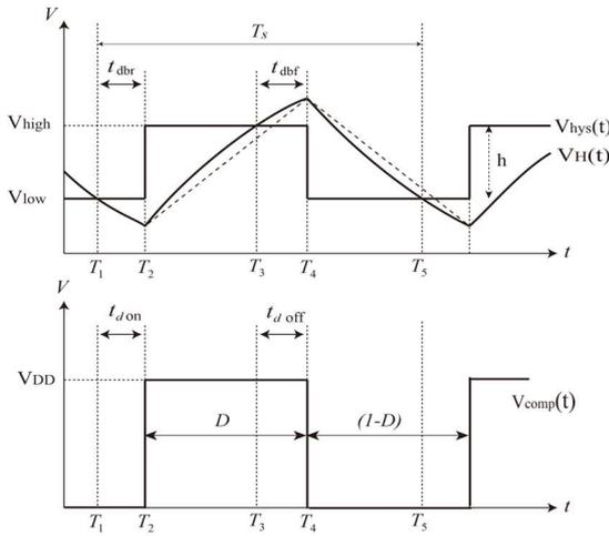
Fig. 2. Input & output waveforms of a hysteretic comparator.
