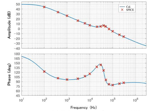
(c)  $V_{out} = 0.9 V, R_{out} = 3 \Omega, f_{sw} = 1.43 MHz$
