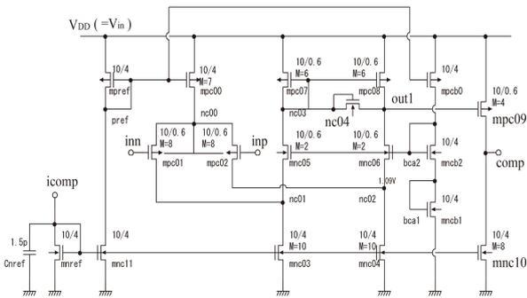
Fig. 3. Designed amplifier circuit used in the hysteretic comparator.
