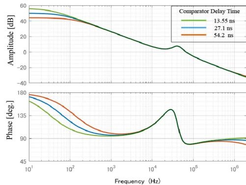
Fig. 8. Bode plot of a hysteretic buck DC–DC converter in varying delay of a hysteretic comparator. (Ideal fsw is 2M\_typ in table 2.)
