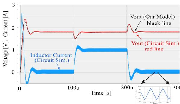
**Fig. 10.** Comparison of the transient at the output with the load current change, and the waveform of the inductor current.
