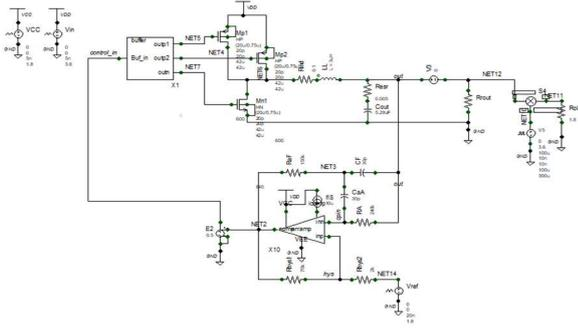
Fig. 7. The SPICE transient simulation circuit based on the use of the designed circuit.
