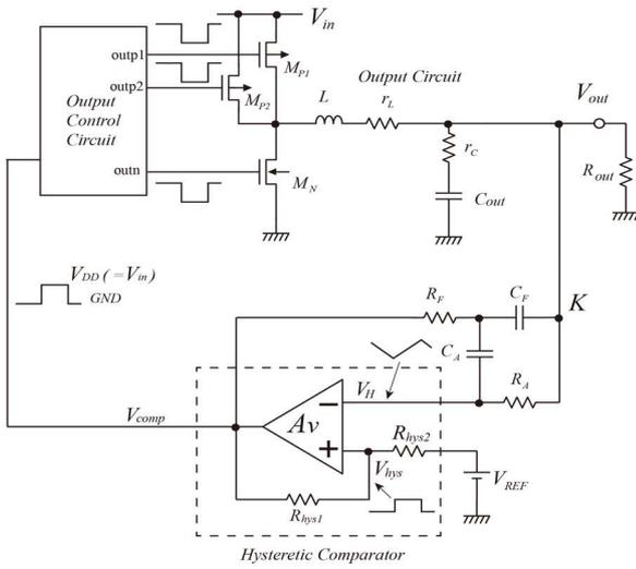
Fig. 1. Hysteretic buck DC-DC converter circuit.
