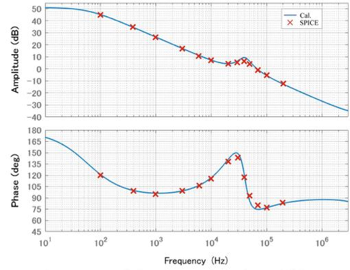
(a)  $V_{out} = 2.7 V, R_{out} = 9 \Omega, f_{sw} = 1.23 MHz$
