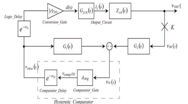
Fig. 5. Small-signal transfer function representation of the circuit in Fig. 1.
