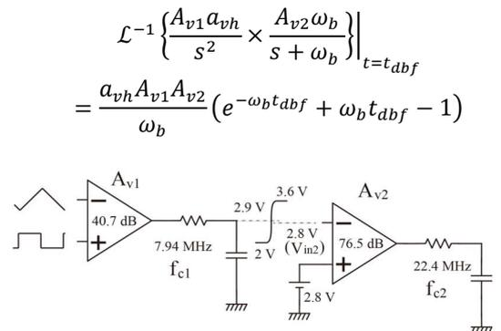
Fig. 4. Internal structure of the comparator in Fig. 3.
