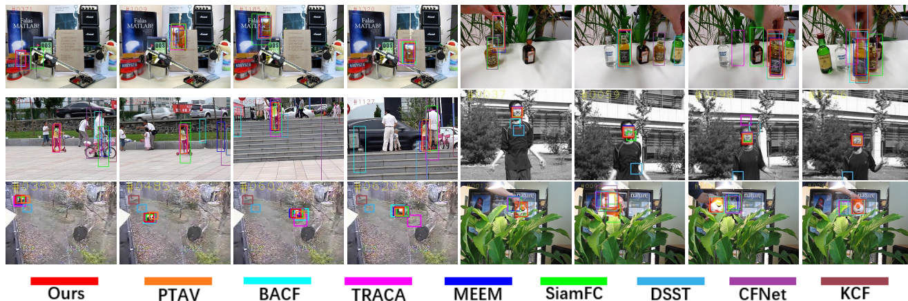
Fig. 11 Tracking results of 9 real-time trackers on 6 challenging sequences from the OTB100 benchmark (from left to right and top to down are Lemming , Liquor , Girl2 , Jumping , Panda , Tiger1 ).
